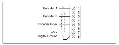
Figure 12. Typical Single-Ended Encoder Wiring Pin Assignment
